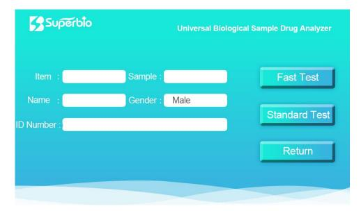
Step 3. Enter the basic information of the suspect and select the type of "Test Item". All the optional test items will be displayed. Select the test type of the corresponding test strip, and select the type of "Sample Type". All kinds of items that can be selected will be displayed. After selecting the corresponding type, the system automatically return to the test interface, and click the "Fast Test" button to start.
