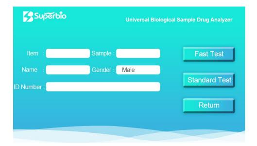
Step 3. Input the basic information, select the test item, click "Standard Test" to enter the test interface. Meanwhile, the instrument starts counting down and waits for the incubation time.
